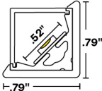
Profile with plastic mounting clip
